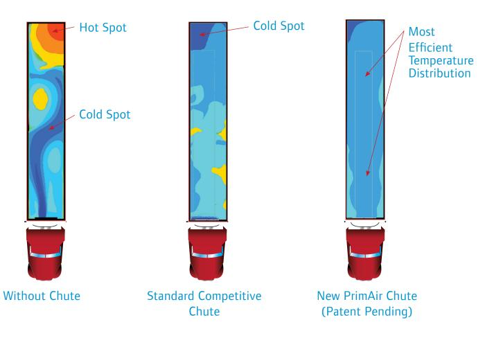
Results based on Thermo King CFD analysis on loaded trailer.
